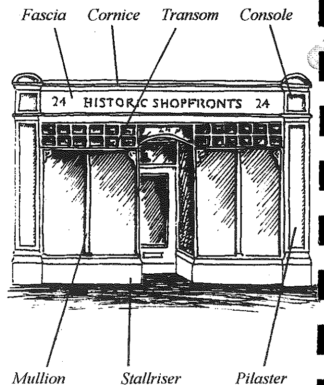
Traditional Shopfront Elements
