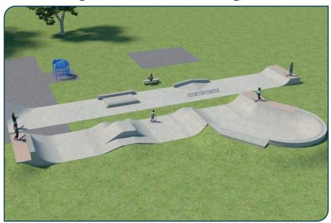
There are limitations to pre-cast concrete layouts so as skate park design evolves, they now use a sprayed concrete method which is hand finished to allow more organic and flexible designs.
