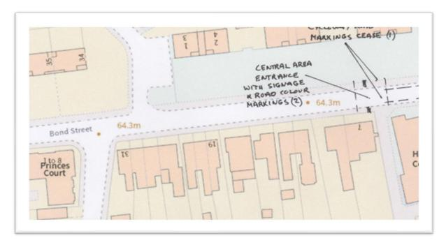
Different road surfacing marks the entry to the central area (2). Signage has been indicated, though this may not be deemed necessary.
