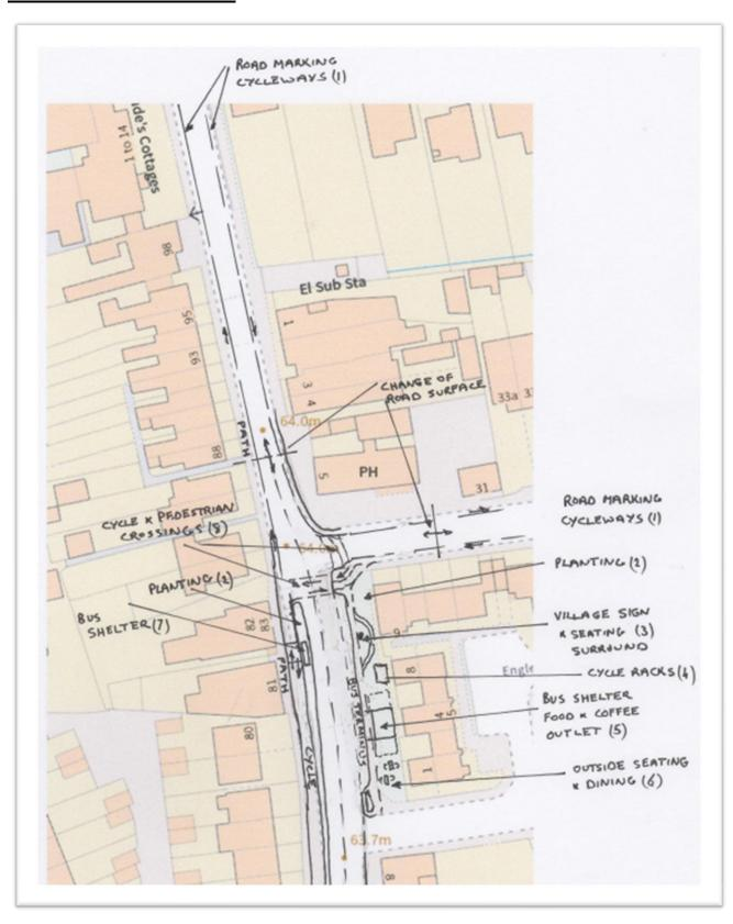
In this section of St Jude's Road, it is proposed to create a small 'transport interchange', taking advantage of the approx. 9m wide by 45m long (currently) area between Alexandra Road and Victoria Street.
