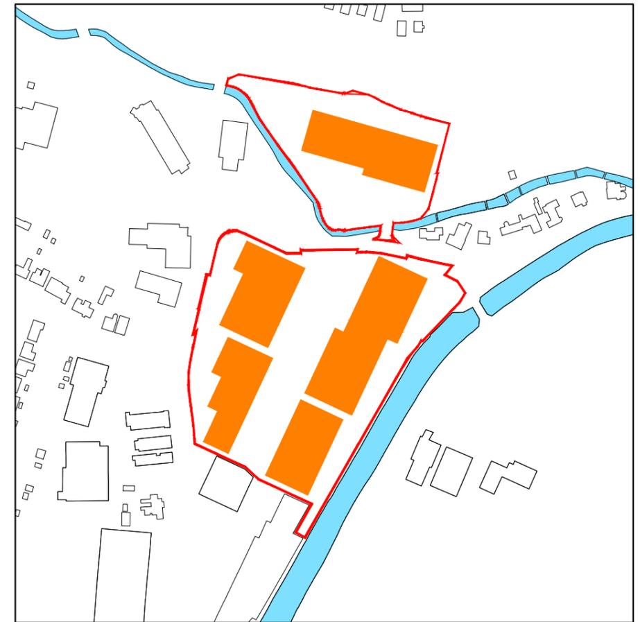
3. The buildings were further stepped and broken up, allowing for setbacks from the site borders. This meant that from the street each unit is perceived as an individual building. The set back from the boundary line also moves the buildings further away from sensitive receptors and creates space for soft landscaping which will help to integrate the proposal into the local context.
