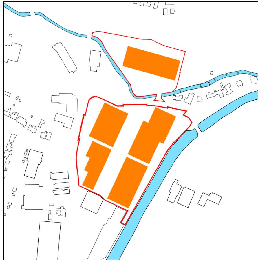
2. The scheme was then divided into smaller building footprints creating breaks in the massing. The stepped frontages staggered the footprint, making the buildings appear smaller overall. Minimising breaks between the multiple units, and creating terraced buildings, allows for efficiency of design with less external walls giving a more efficient and sustainable building fabric.
