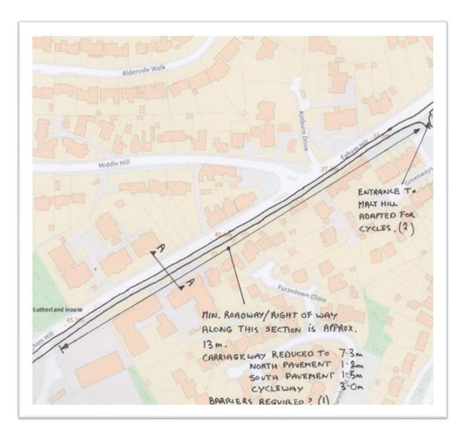
This section is the narrowest and requires a reduction in carriageway width to 7.3m. Road colour can be changed, and other visual means used to make vehicles aware, (and a 30mph speed limit throughout the length of Egham Hill is assumed)
