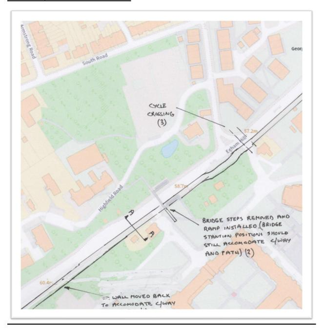
The verge along this section gradually narrows from the footbridge to the traffic lights and a section of RHUL wall will need to be moved back to accommodate the cycleway/footpath (1)
