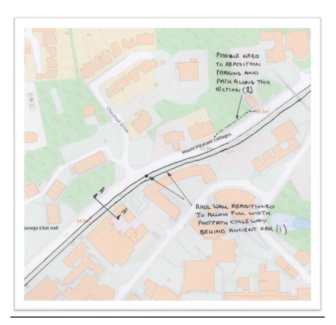
There are few obstructions to the new format along the first part of this section, though there is an ancient oak tree opposite Chestnut Drive, and the cycle way and footpath need to go behind this tree. The RHUL wall will have to be moved back to accommodate this.
