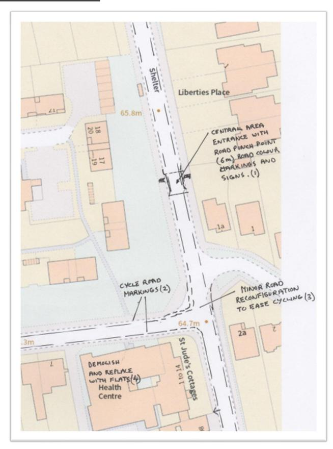
It is proposed that the North End of the designated Central Area is placed a short distance past the junction of St Jude's Road and Bond Street. This would be marked by a pinch point in the road width to 6m (currently approx. 7 m), road surface change and entry signs (1). Cycle way would pass behind the pinch points (see example below)
