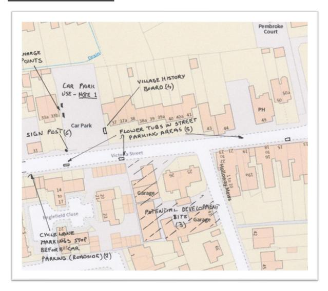
The problem of on street parking versus cycle lanes occurs at the top of Victoria Street (2), but it is felt that Cycling in this road will be relatively safe with a 20mph speed limit and relatively low traffic volumes.
