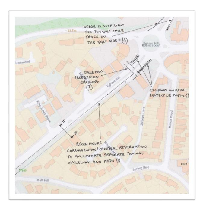
The last section of Egham Hill is relatively straight forward, though the inclusion of the cycleway will require the East side of the dual c/way to be single track and the entry and exit from the garage will need to be reconfigured. (1)
