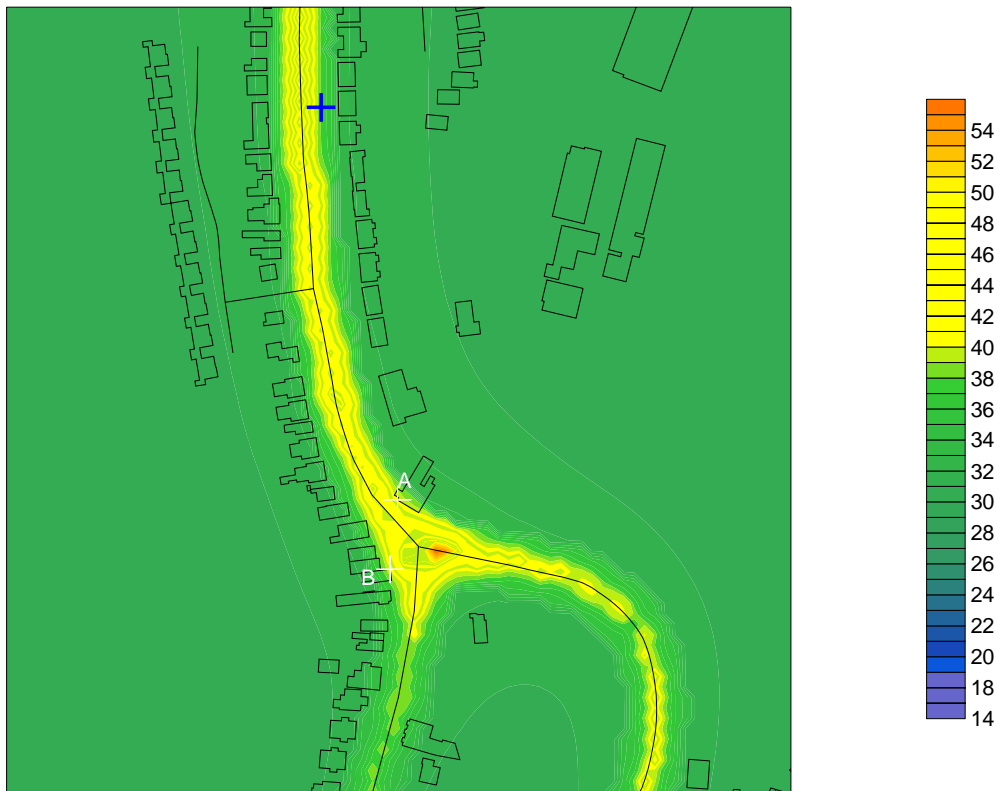
Figure 5 Predicted annual mean NO 2 (µg m -3 ) at New Haw for 2005 base case (with 2003 meteorology)
